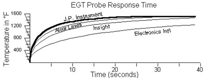
The reduced size of the **JPI Hastaloy-X-tip probes produces faster response** and more accurate than the massive factory installed probe. Therefore **JPI** probes may read as much as 100°F higher than the factory installed probe. However, note that the engine was certified with
