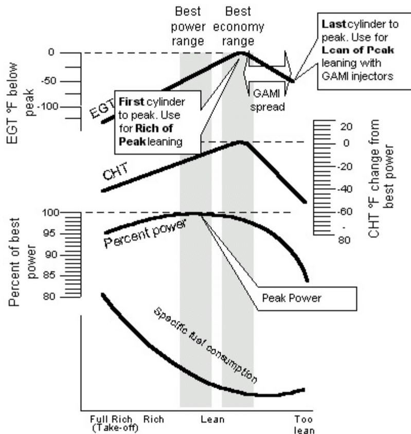
As the mixture is leaned, EGT rises to a peak temperature, and then drops as the mixture is further leaned. Peak *power* occurs at a mixture using more fuel than at peak EGT. Best *economy* occurs at peak EGT. Accurate leaning yields optimal engine temperatures. By being able to precisely adjust the mixture, your engine can produce either the best fuel economy or maximum power, whichever you choose.
