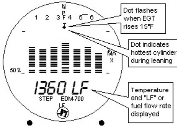
Continue leaning slowly. With a vernier mixture control, turn the knob about a quarter turn every second. With a non-vernier or quadrant mixture control, lean slowly and smoothly about 1/16 inch every five seconds. Eventually, one cylinder will reach peak before any of the other cylinders. The EDM will determine this automatically. *Notice that this cylinder does not necessarily have the hottest EGT.*
